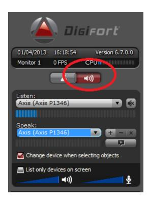
The system allows the creation of groups of audio output devices, this way, the operator can send audio to many cameras simultaneously:
