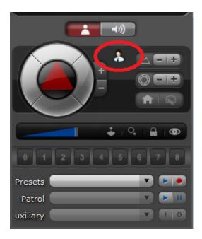
By pointing the mouse button over the icon, the operator will have details of who is using the camera PTZ:
